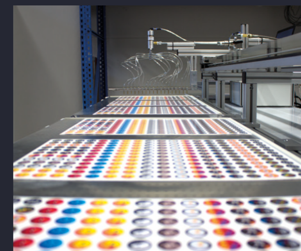
3D-Aufkleber-Domingleistung: ca. 24.000 St./Std. (Ø 20 mm) 3D sticker doming performance: approx. 24,000 pcs./hr. (Ø 20 mm)
